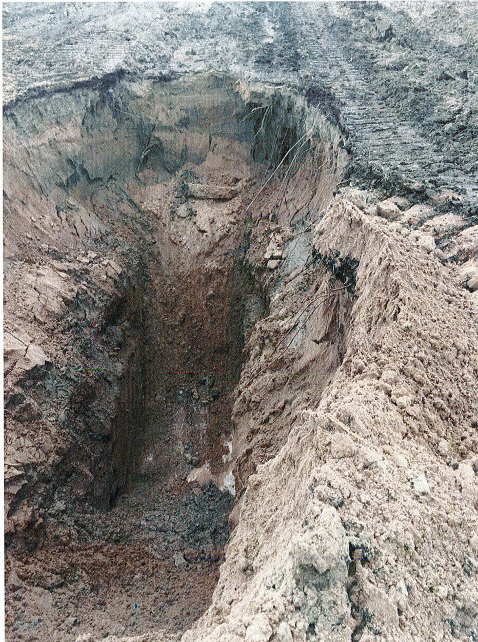
Photo 1: Test pit for cap material
