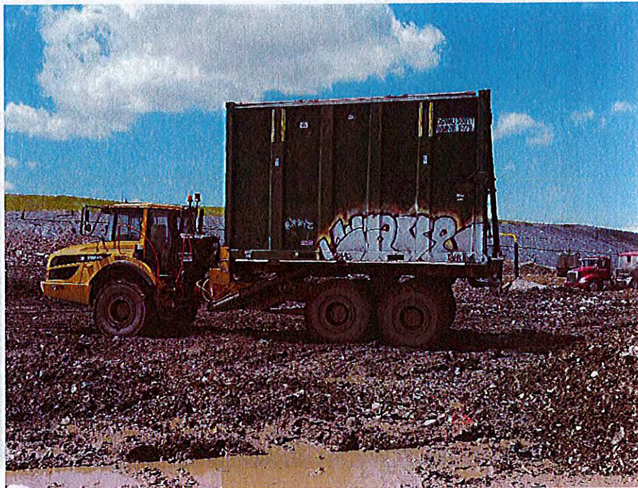
Photo 13 – Rail Container Being Transported to Active Region of Cell 12 to be Unloaded
