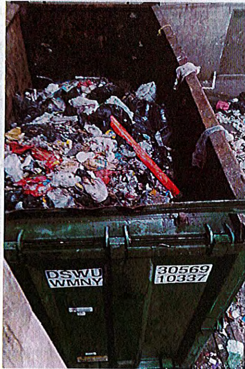
Photo 8 – Temperature Probe Placed in Center of Rail Container WMNY 10337
