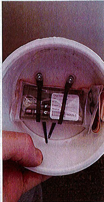
Photo 1 – Cargo Data Logger Unit Installed Within PVC Cap
