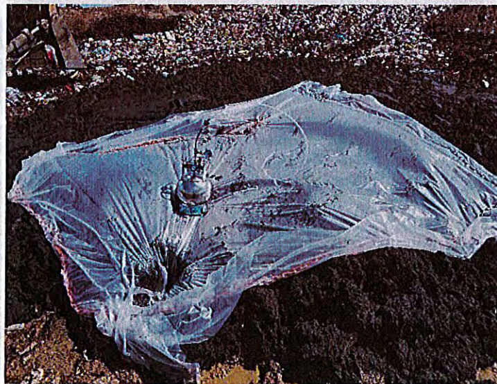
Photo 34 – Silonite Can Setup – Bio-Solids Pile
