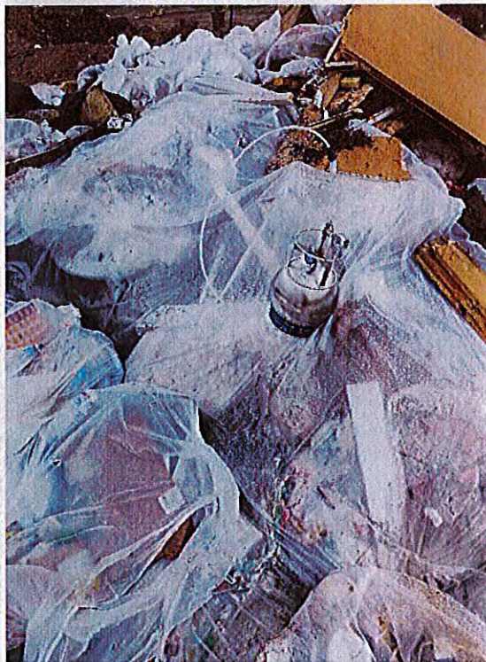
Photo 28 – Silonite Can Setup – WM Local Front Loader Waste Pile
