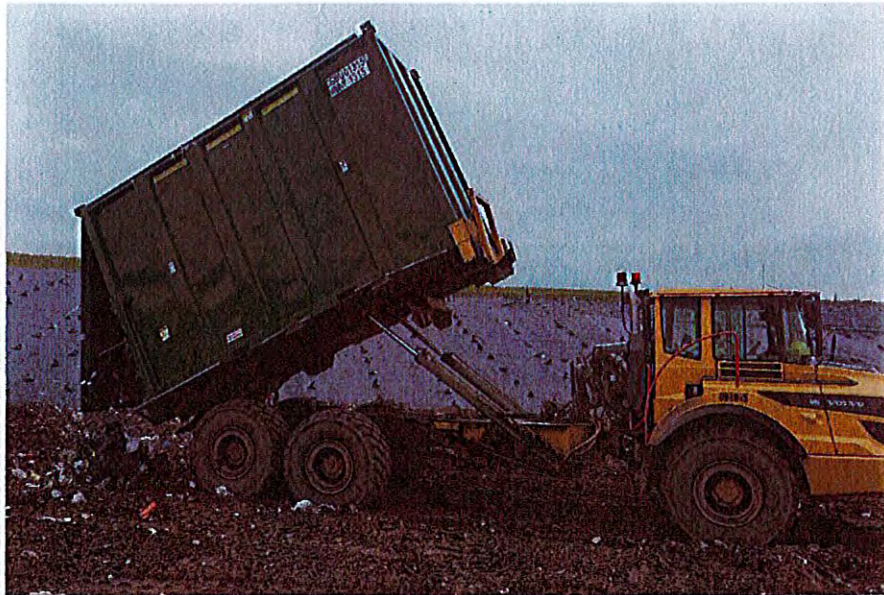
Photo 115 – MTS Southwest Rail Container WMNY #1315 ready to be unloaded in Cell 12
