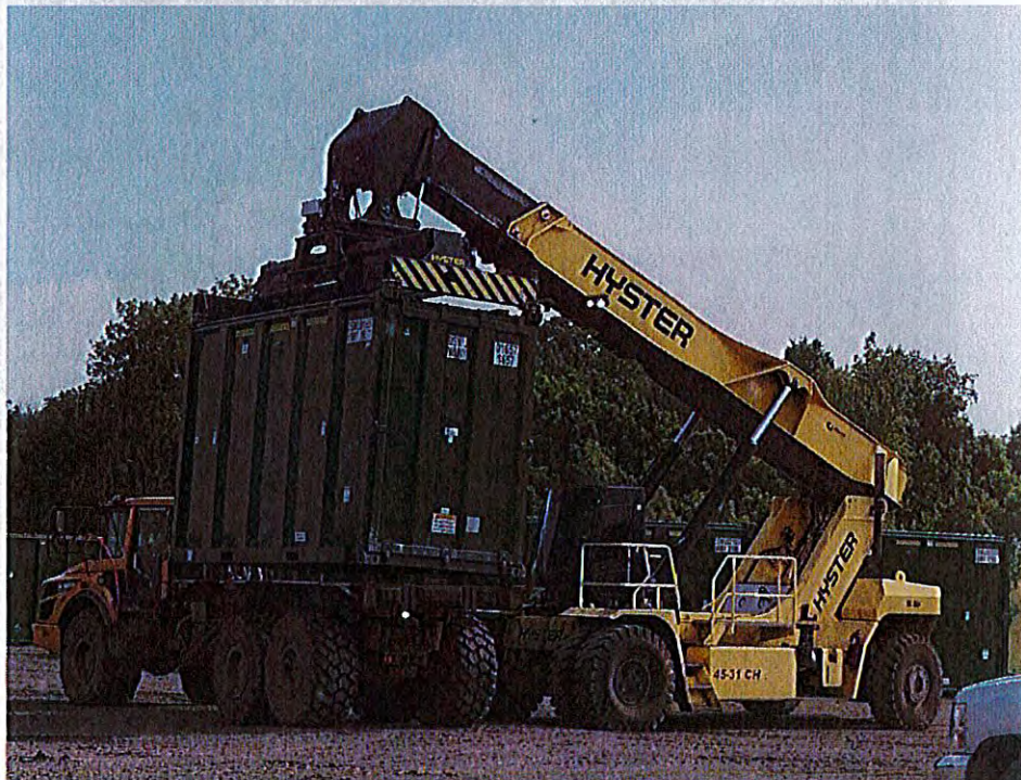
Photo 130 – MTS Southwest Rail Container WMNY #1657 being hoisted onto transport vehicle
