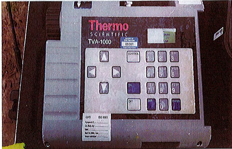
Photo 35 – TVA-1000 Unit Used for Rail Container Gas Monitoring
