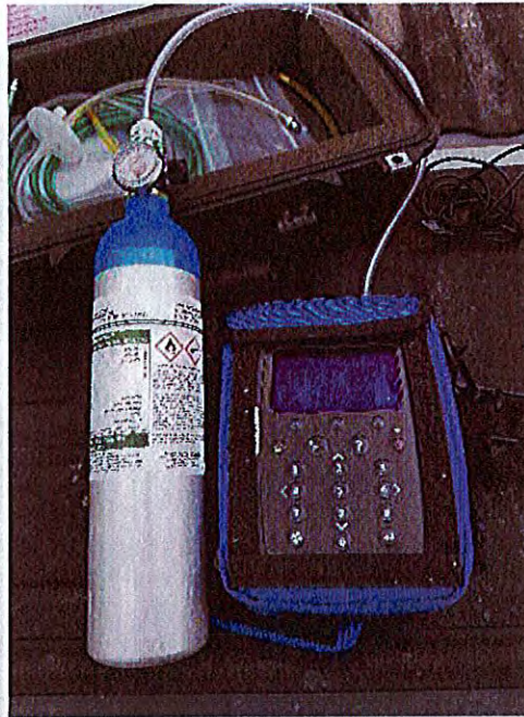
Photo 37 – Landtec GEM-5000 Unit used for Rail Container Gas Monitoring
