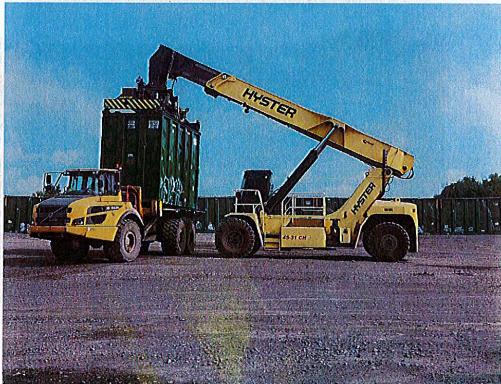
Photo 136 – MTS Hamilton Rail Container WMNY #0122 being hoisted onto transport vehicle
