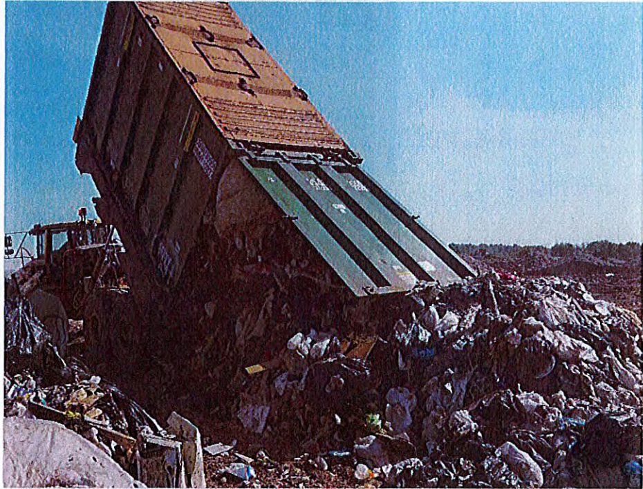
Photo 105 – Review Rail Container WMNY #10337 being unloaded in Cell 12
