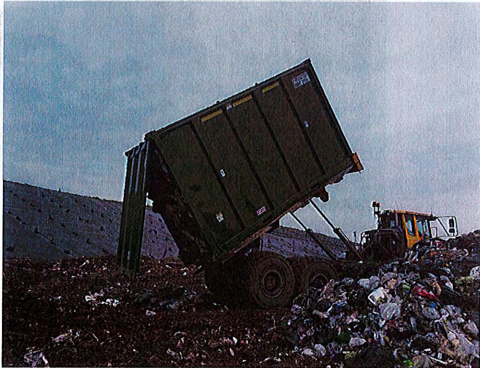
Photo 124 – MTS Hamilton Rail Container WMNY #2109 ready to be unloaded in Cell 12
