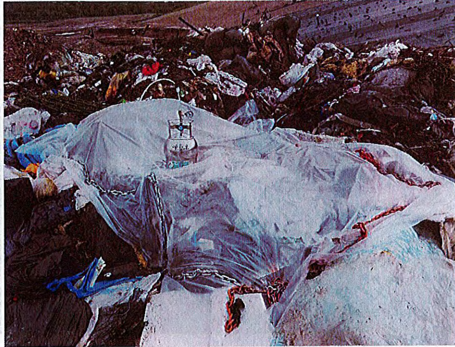
Photo 23 – Silonite Can Setup – WM Local Rear Loader Waste Pile
